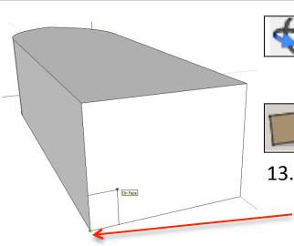
12. Use *the orbit tool* to rotate the boat so you can see the rear of it.
